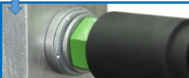
Guide the bolt and the collapsible washer through the pre-drilled hole of the connection, it is advisable to hold the split washer as it enters the pre-drilled hole. Make sure the holes are aligned properly.
