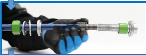
Un-assemble the ONESIDE. Sliding the components back onto the shaft of the tool.
