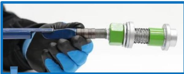
Slide the sleeve back on the tool and insert the tip of the bolt into the socket. To lock the ONESIDE to the tool, slide the sleeve forward.
