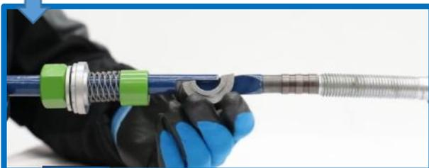
Move the split / collapsible washer to the correct seating location on the tool and fold as shown. It is important the split washer is seated correctly. Now the ONESIDE is ready for installation.
